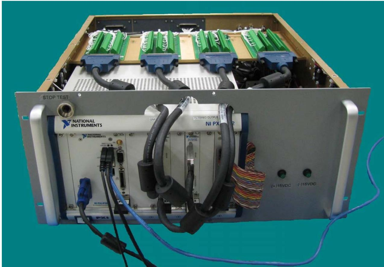
*The IWS is a PXI based data acquisition system that is designed to receive 16 or 32 strain gage inputs from 1 or 2 train car wheel sets. The inputs are combined using algorithms to provide outputs that are a measure of various combinations of vertical, lateral, and longitudinal forces on the wheels.*
