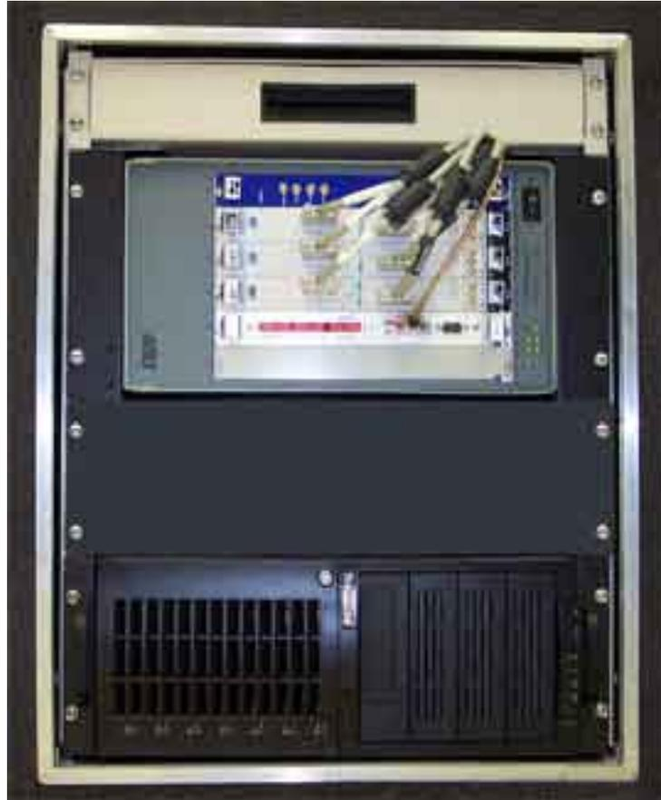
*Complete Network's High Speed Data Acquisition System is a state-of-the are solution for acquiring and recording 24 analog channels and converting them to digital using VXI Technology's 1433B Sigma Delta Analog to Digital Converters. With 16-Bit resolution and 196 KiloSamples/per second/per channel, the HSDAS represents cutting edge technology that delivers solid performance. The HSDAS features a user-friendly graphical interface and real-time displays of each individual channel.*
